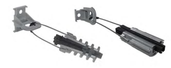
**Appointment:** Designed for anchoring the insulated load-bearing conductor SIP-2 on end, corner and branch supports. Fixing to the poles is carried out with screws or with an F 20 mounting strap. Anchoring clamps can be supplied in versions with a cast body or with an extruded profile body. The "N" version is equipped with a stainless steel cable.
